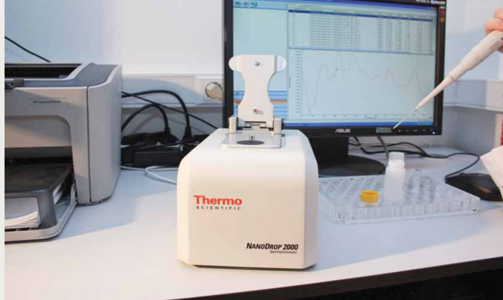
Fig. 4. ND-2000 NanoDrop spectrophotometer (photo by G.N. Dudchenko)
