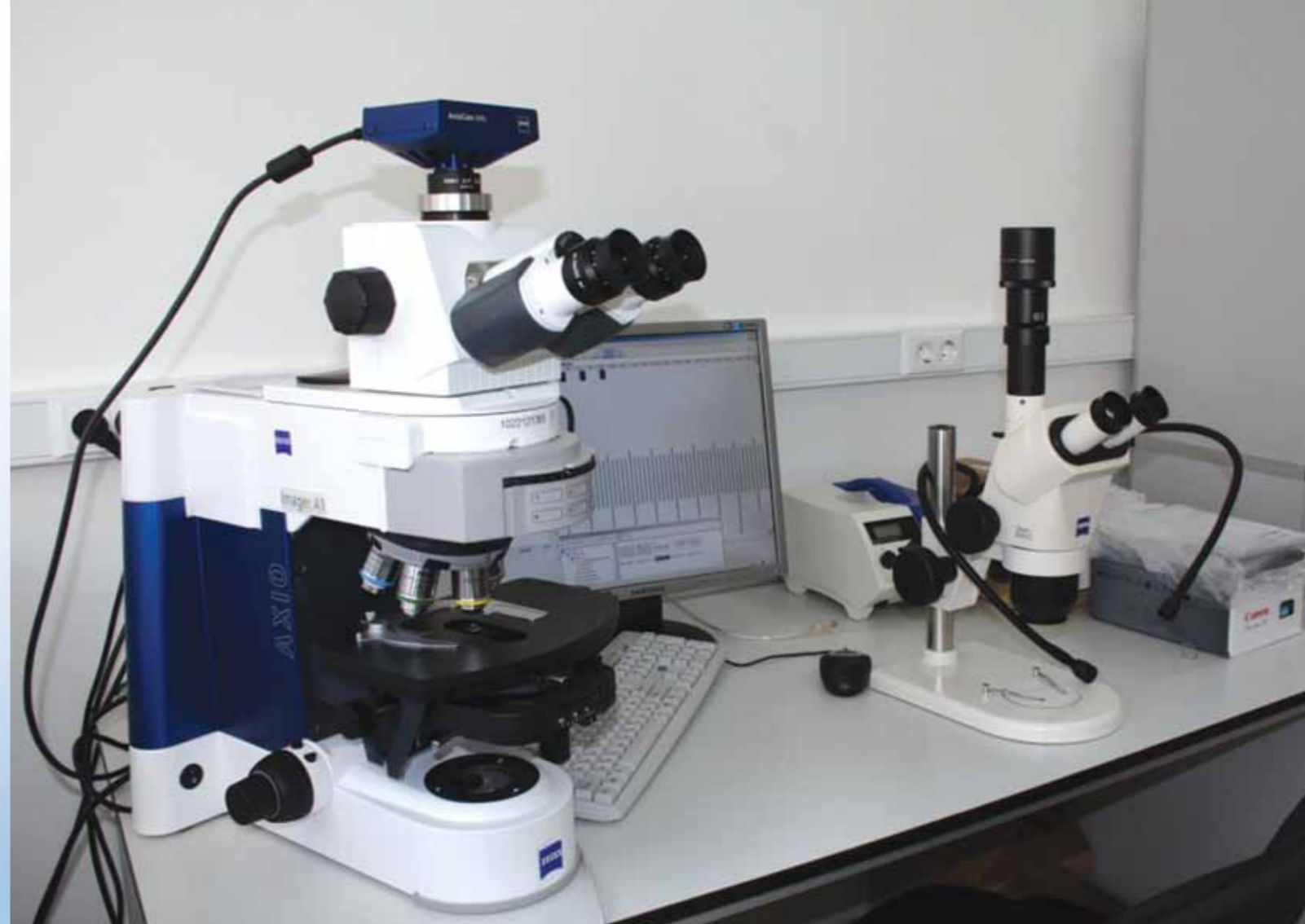
Fig. 2. Advanced optical instruments: Zeiss Axio Imager A1 optical microscope and Stemi 2000C stereoscope (photo by G.N. Dudchenko)
