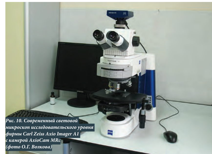
Fig. 10. Advanced research light microscope by Carl Zeiss Axio Imager A1 with a AxioCam MRC camera (photo by O.G. Volkov)
